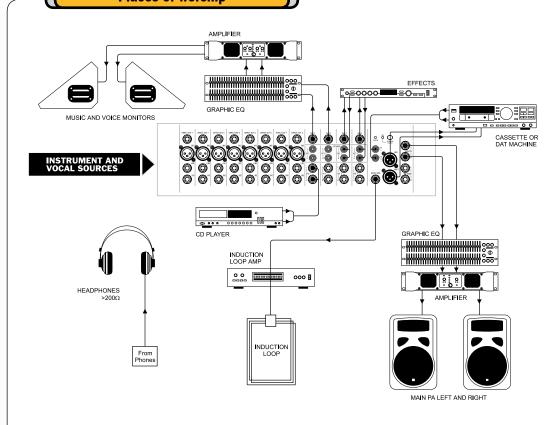
With the M Series mixer configured as shown in this diagram, it will provide a mono output to feed the main PA system, with an induction loop added for the hard of hearing. For larger scale occasions, music and voice monitor mixes may be required, which can be sent via the auxes. The main stereo mix output can also be sent to a 2-track recorder, such as a cassette or DAT recorder, if the occasion is to be recorded.
